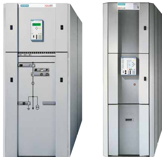
Fig. 2/16 Left: switchgear with numerical relay (7SJ62) and traditional control; right: switchgear with combined protection and control relay (7SJ64)
