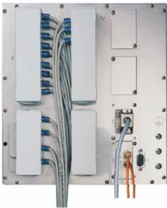
Fig. 6/51 Rear view with terminal covers and wiring
