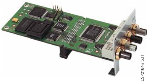
Fig. 6/64 PROFIBUS fiber-optic double ring communication module
