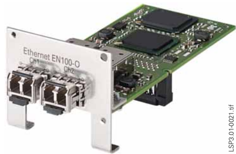
Fig. 7/63 Fiber-optic Ethernet communication module for IEC 61850 with integrated Ethernet switch
