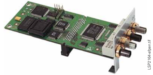
Fig. 7/21 PROFIBUS communication module, optical double-ring
