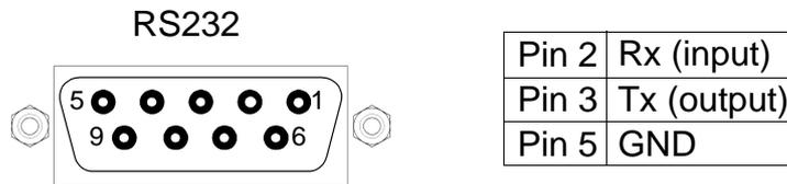
Figure 18 DSUB–socket at the CC–2M
