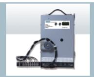
The communication module is the interface used to connect the MJ-4A & MJ-4B control panels to SCADA. The RS232/485 connection supports RS232 multi-drop configurations and RS485 loop, star and open end configurations. The fiber optic ST connections supports a loop or star configuration. The communication module can be preinstalled in the control panel or easily retrofitted in the field.
