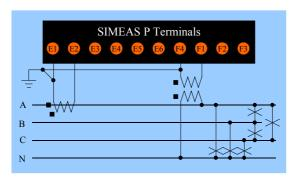
Four-wire three-phase, unbalanced (low voltage system)
