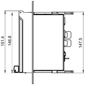
Housing: Panel flush mounting or cubicle mounting 5-7/8" x 5-7/8" (138<sup>+1</sup> x 138<sup>+1</sup> mm) Panel section: Protection Class: Front IP 41 or IP 54 (refer to ordering
