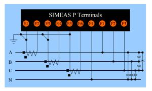
Four-wire three-phase, unbalanced (high-voltage system)
