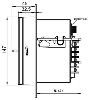
Width of the device: 144 mm
