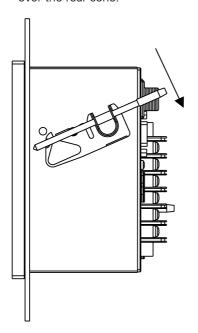
Note: Minimum thickness of the mounting plate: 1 mm; steel
