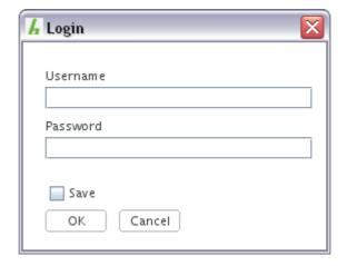
For devices connected via TCP/IP, usually login credentials are needed. If they are not yet stored or not valid anymore, a dialog is displayed which allows input of username and password. In case of a *hopf 7050RC* network management card either the users *master* or *device* are allowed. The password matches the password configured via the Web-Interface or the *Network Management Assistant*.
