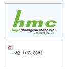
The device is logically presented as a sub-element of the *system overview node*. In this case, the device has no sub elements of its own. Yet this is possible, as can be seen in case of the *hopf* 7001RC. The device's id and port name are presented dark grey and bold. This, like the icon ✓o, means that the device is connected. In the device's context menu, to be activated by right-clicking the device in the tree, as well as in the menu *Devices*, there is a menu item *Disconnect*.
