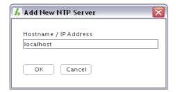
After entering a host name or IP-Address and confirming with the OK-Button a new Tab is added to the NTP panel.
