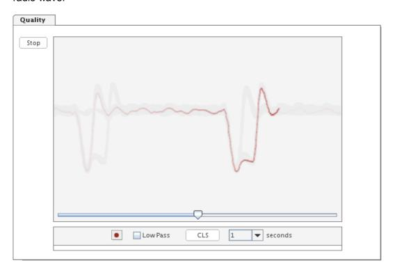
This signal, generated and emitted via radio in Braunschweig, Germany, transmits bits of information encoded as shorter and longer (typically 100ms and 200ms) signal level drops. The falling flank of these level drops signifies the exact second change. The Image shows more or less the ideal case of such a signal that is realized by connecting the DCF77 input to the DCF77 simulation output of another device, instead of to an antenna.
