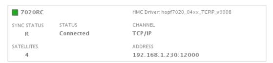
The left hand area shows synchronization and connection status and, in case of a device equipped with a GPS receiver, the number of tracked satellites. The right area contains the driver identification the device is logically integrated with in the HMC, as well as an indication of communication channel and connection settings.
