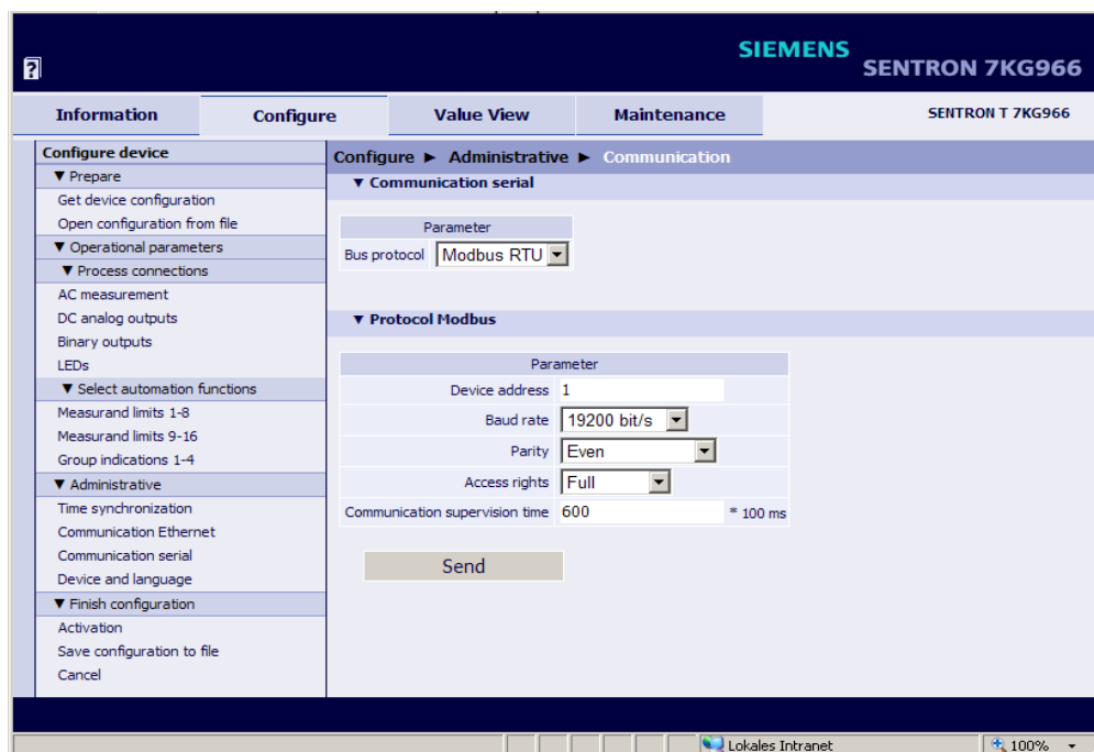
Fig. 7-38 Configure Tab, Communication Serial via Modbus RTU Input/output Window
