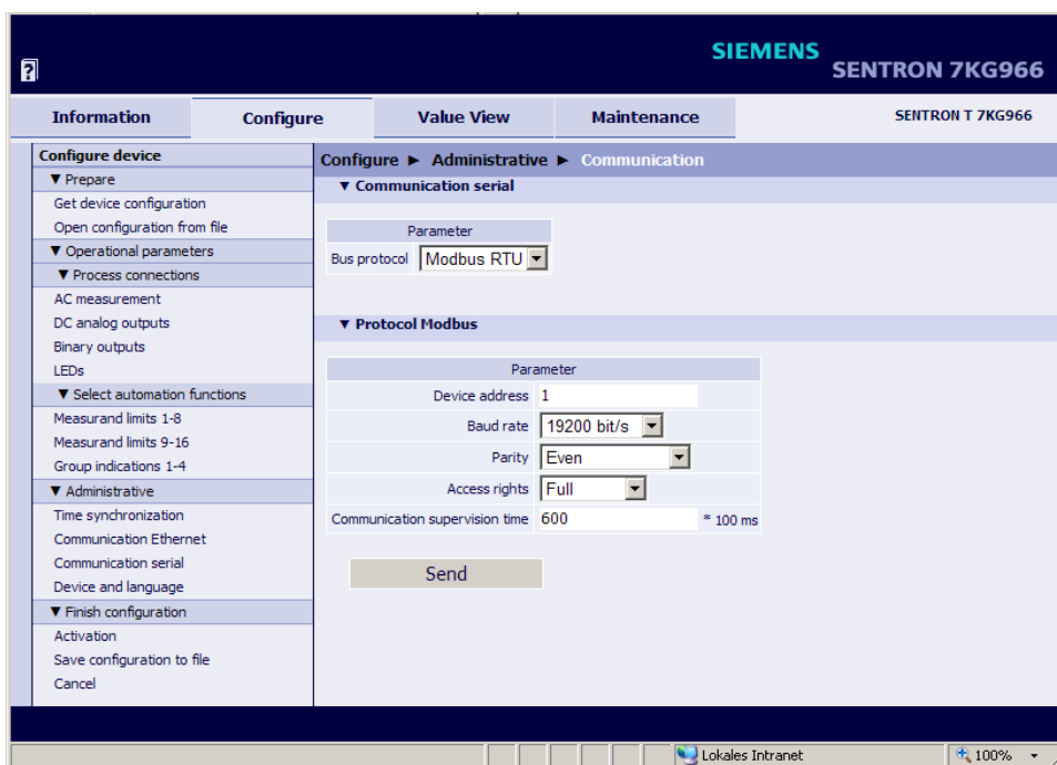
Fig. 7-59 Configure Tab, Example of Serial Communication Settings
