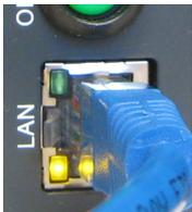
At the *LAN* terminal, *SIMEAS Q80 7KG8080* is connected with the Ethernet and the PC. For connection via a local network, an uncrossed Ethernet cable must be used, and for direct connection of the measurement device to the PC, a crossed Ethernet cable is required.
