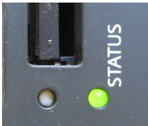
The *STATUS* LED indicates the device's current operating status. Right after the device is activated, it flashes red a few times, then proceeds to flash green (during which the memory card is checked for any available measurement task to start) and finally goes off, which is indicative of normal operation..
