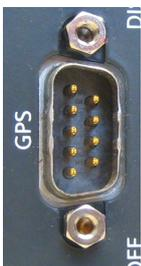
At the nine-pin GPS socket it is possible to connect a **GPS-receiver** of the type e.g. **Garmin GPS18LVC-5Hz**, **Meinberg GPS161AHSx** (item number: 25150) or **HOPF6875** (from firmware 7.0, order number 7XV5664-0CA00). This enables absolute synchronization to GPS time. If the GPS-receiver has reception, the measurement system synchronizes itself automatically. Find more information about setup and configurations in section Synchronisation of several devices.
