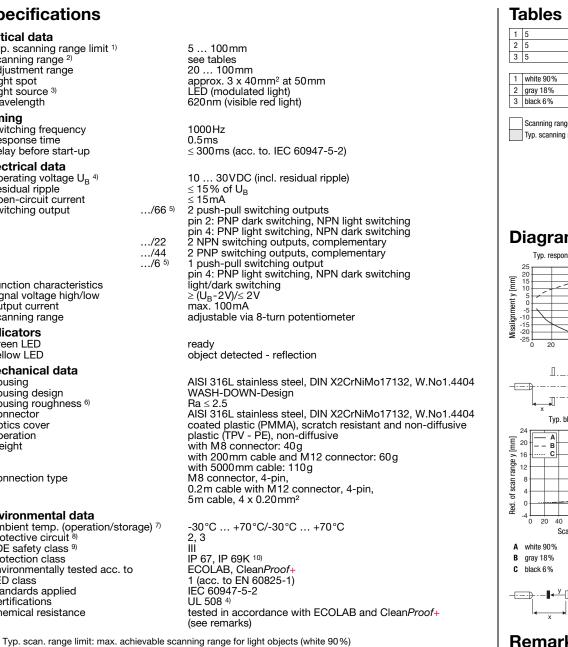
Scanning range: recommended scanning range for objects with different diffuse reflection 2)
