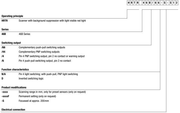
N/A Cable, standard length 2000 mm ,200-S12 Cable, length 200 mm with M12 connector
