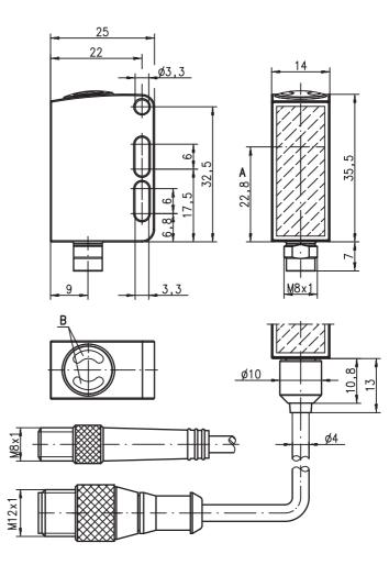
Optical axis Α в Indicator diode
