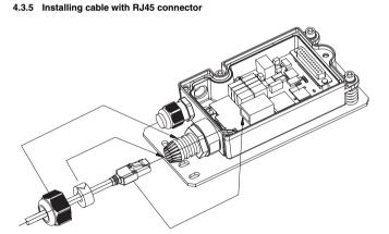
Figure 4.7: Installing cable with RJ45 connector
