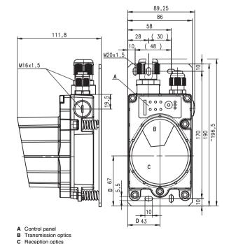
Figure 2.1: Dimensioned drawing of DDLS 200 Ethernet version for cable with RJ45 connector
