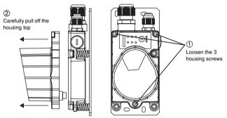
Figure 3.3: Removing the housing top
