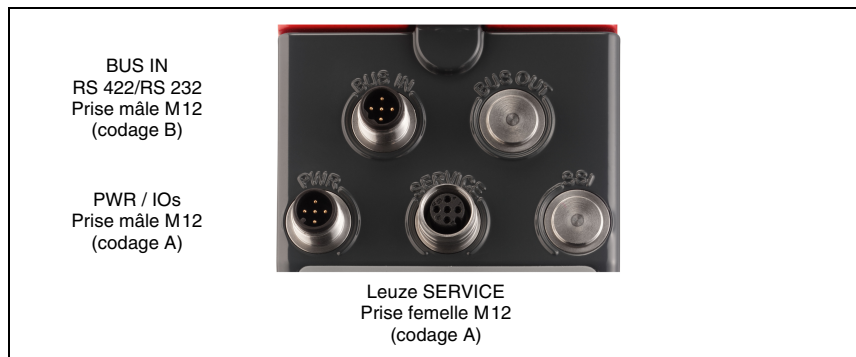
Figure 7.1 : Raccordements de l'AMS 300 i
