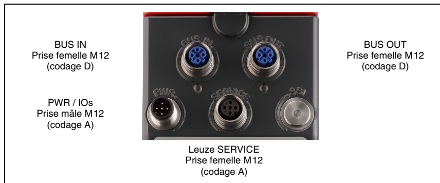
Figure 7.1 : Raccordements de l'AMS 308 i
