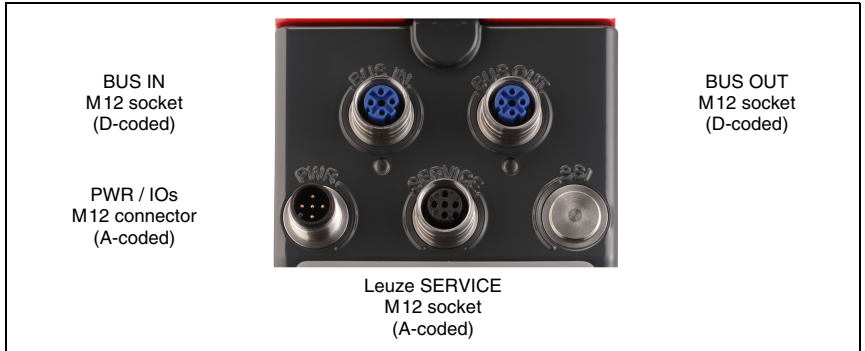
Figure 7.1: Connections of the AMS 348 i
