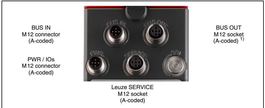
Figure 7.1: Connections of the AMS 355 i
