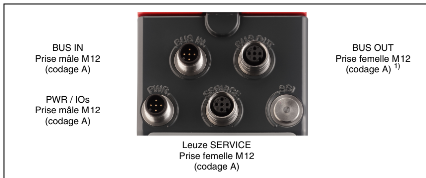
Figure 7.1 : Raccordements du AMS 355 i
