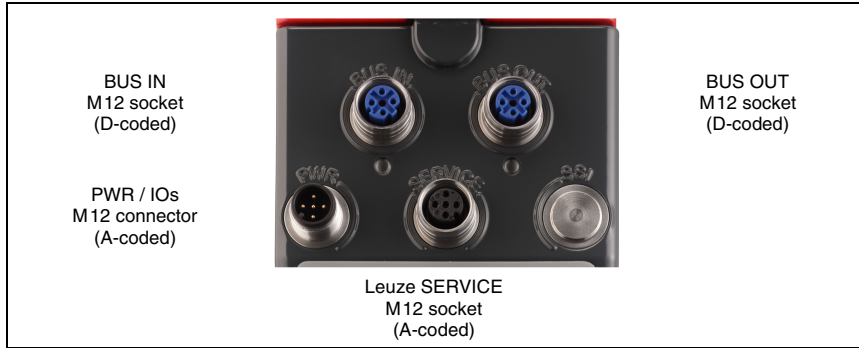
Figure 7.1: Connections of the AMS 358 i
