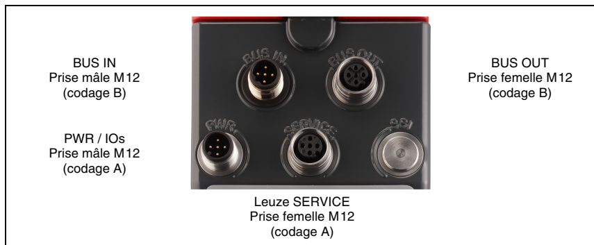
Figure 7.1 : Raccordements du AMS 384 i
