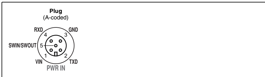
Figure 3.3: BPS 8 - assignment M12 connector PWR IN
