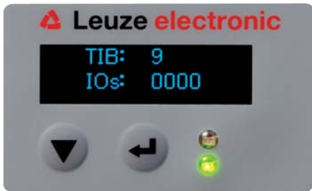
Figure 8.3: Display showing the measurement operation state of the light curtain
