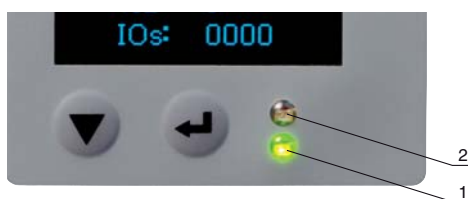
Figure 3.2: LED indicators on the receiver
