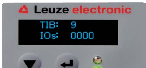
Figure 3.3: OLED display on the receiver
