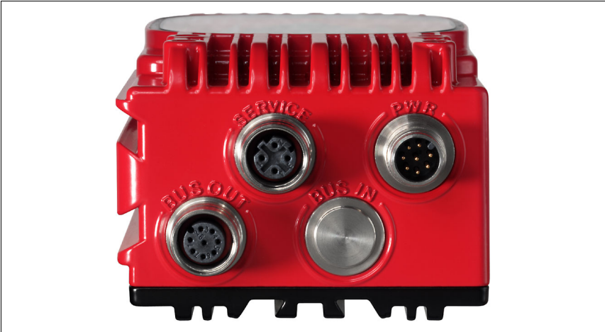
Figure 5.1: Location of the electrical connections
