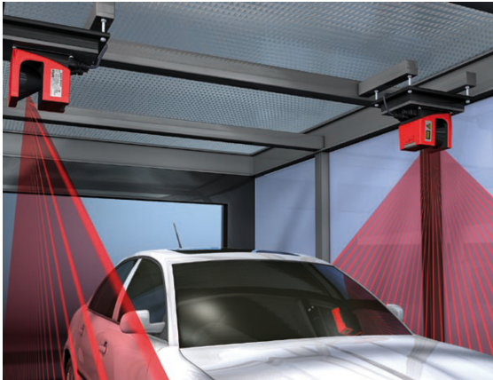
Figure 3.8: Application example - automatic parking system
