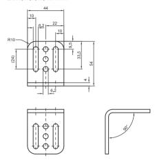
Fig. 12.2-3: Standard mounting bracket
