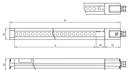
Fig. 12.2-1: Dimensions Safety Light Curtains
