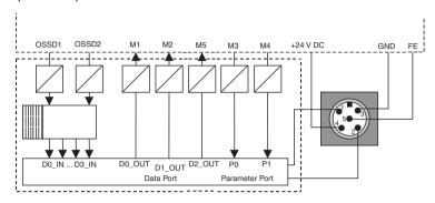
Fig. 7.9-5: Machine interface /A1, schematic structure
