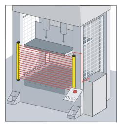
Fig. 3.4-1: COMPACT plus-b Safety Light Curtain – Application for a press
