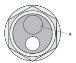
a = Just push opening through when a separate connection cable for the load circuit is to be connected.
