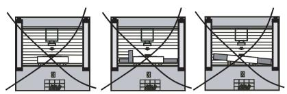
Fig. 4.3-2: Shadows in the protective field must always be prevented.
