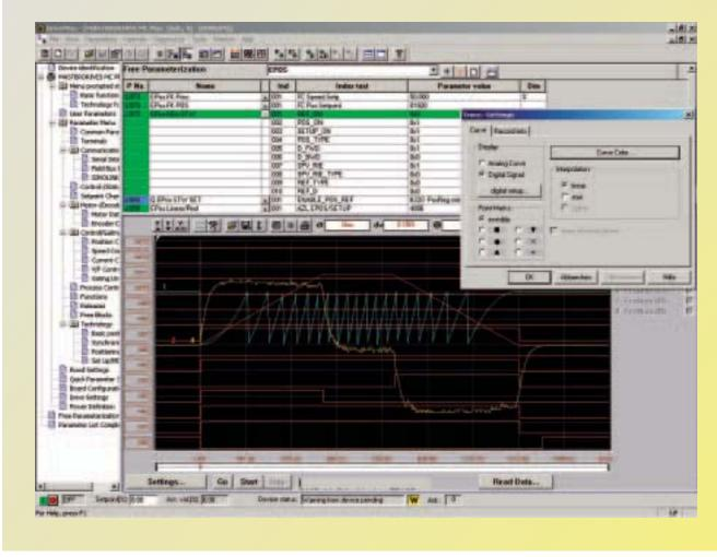
Fig. 2/11 Trace Function with DriveMonitor
